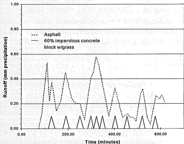
Figure 3. Runoff volumes from asphalt and permeable pavements.
