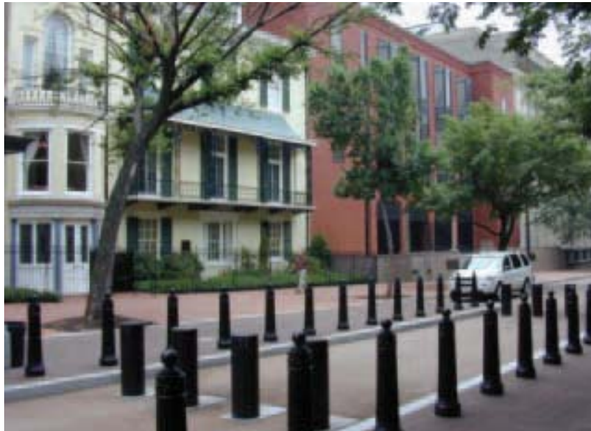
Historic properties often cannot meet setback requirements. Limiting street access by using appropriately designed concrete barricades is one solution for medium- or high-risk buildings located close to sidewalks. The Madison House is located close enough to the White House to require more extraordinary security measures than other historic properties.
